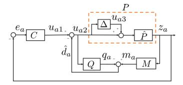
Fig. 4. Closed-loop system with DOB incorporated.
