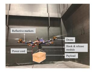
**Fig. 8.** Experimental platform: the drone is connected with a thin light power cable and its influence to the results are negligible. The cable is placed at the same position for each test. A bottle of water is used as the payload in the real test and the payload weight is changed by adding/reducing water in the bottle.
