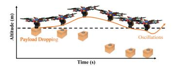
Fig. 1. Oscillations during payload dropping.
