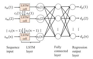
Fig. 11. LSTM network structure.
